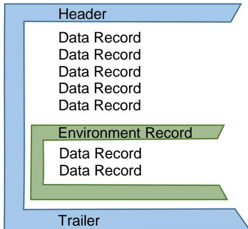
Figure 2: No Encryption FI and one Environment FI
